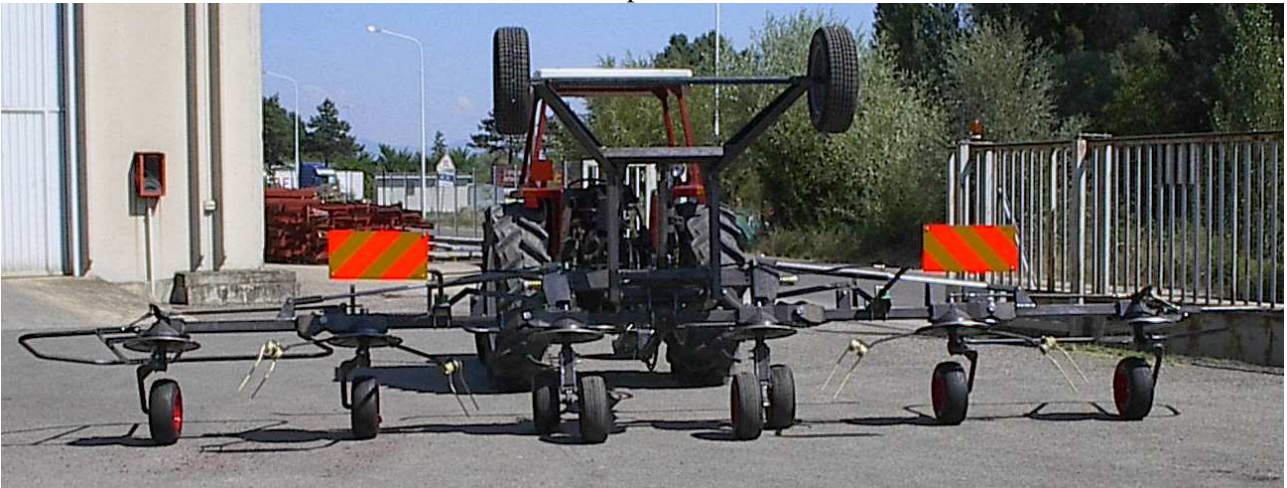
Fig. 2 - Use the pivot (3) and the elastic pin (13) to assemble the rotor group. Now assemble the transport axle with the pivots (5). Use the grommet nuts (15) to fasten the wheels on to the rear axle.
